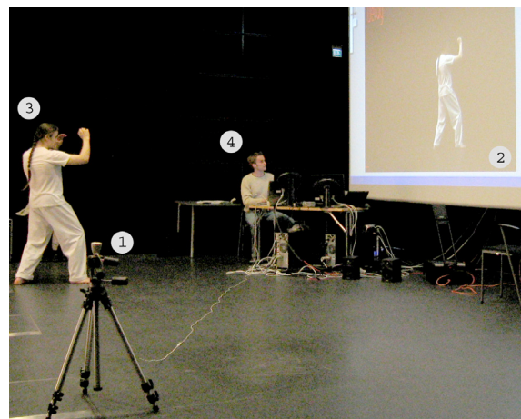
Figure 1. Test setup, showing camera (1), camera view projected on a screen (2), user (3) and test instructor (4).
