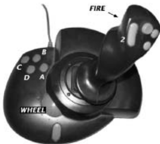
Fig. 7. The joystick's stick, fire button, button 2, wheel, and base buttons (A, B, C, D).
